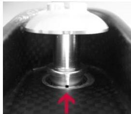
Do not remove the screw over this limit in order not to damage the seat pin of the limbs: this damage nullify the warranty.
