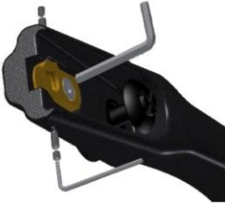
The alignment of the limbs can be done with **bow unloaded**, operating the two side grains, after removing the two locking grains and slightly loosening the central screw. When alignment is done, tighten the grain on the opposite side of where you last worked, re-insert and tighten the locking grains and the central screw.
